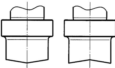
3.) rooftop shear or inverted rooftop shear
