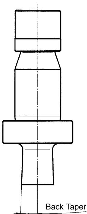
However it should be mentioned that back taper is very important when punching materials such as Stainless Steel or very thick material to reduce galling and eliminate breakage of the tool corners and edges.
