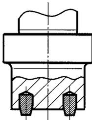
1.) Punch with rubber ejector pin
