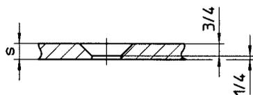
2.) The max. depth of a 90° sunk is 3/4 of the sheet thickness as the entire material thickness cannot be punched.
