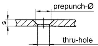
1.) In order to make deformations (material deformations) it is necessary to pre-punch the clearance hole. This pre-punch is normally bigger than the finished clearance hole.
