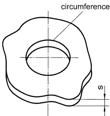
$$F \text{ (in kN)} = \frac{U \times s \times R_m \times 0,9 \times f}{1000}$$
