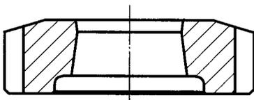
2.) Dies in slug-trap version (negative cutting-edge, to trap the slug).
