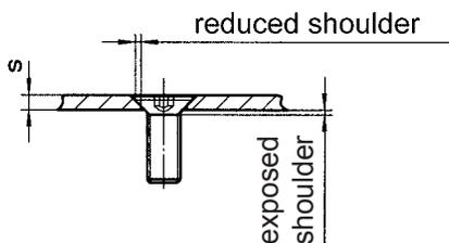
a.) A bigger screw thread clearance hole than required. Keep in mind that the surface area for the head support is reduced and the strength calculation must be adjusted accordingly.
