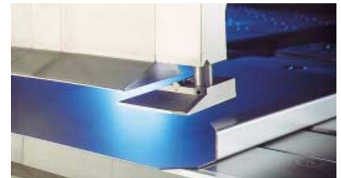
Tabs used for spot welding are easily done with **specialized RAS tab tools**. The robotic tool changer places them at any position along the working length.
