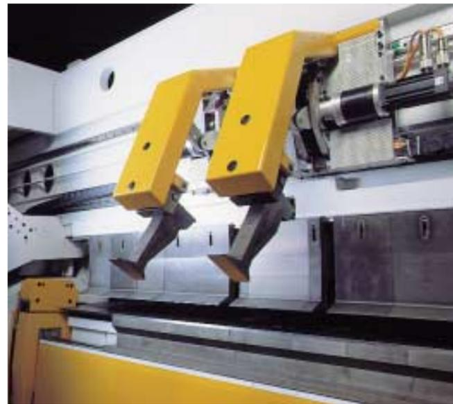
The **segmented folding beam tools** offer even more design flexibility, if window bends, tapered parts or offset bends are required. Using basic segments and adapter pieces any tool length can be set up.
