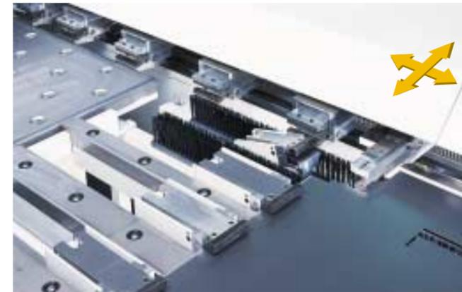
The "Magic-Eye" system scans the notch and/or edge of the blank.
