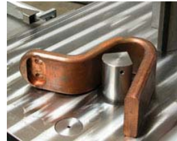
bending of round stock copper
