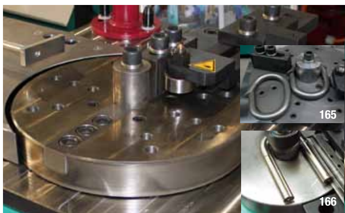
164 Standard Drehteller ø390 mm Standard round table ø390 mm
