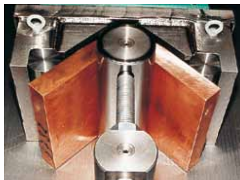
78 Dicke Platten biegen CU 300x40 R=40mm Bending huge flat material
