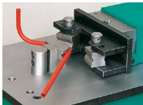
75 Hydraulikrohr biegen Hydraulic pipe bending
