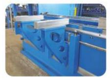
Moveable heavy-duty front supports on linear guide
