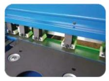
Specially-designed rectangular hold downs, suitable for cutting narrow stripes (optional)
