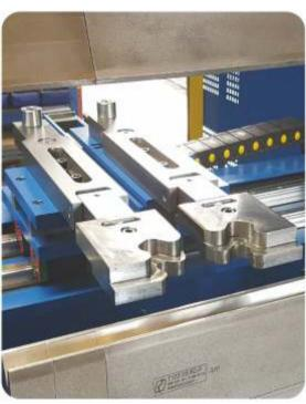
Specially designed finger stops offering high accuracy and maximum flexibility even in conical bends. Maximum stop position 1200mm
