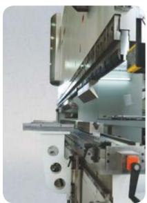
Heavy-duty clamping system up to 350t/m (optional)
