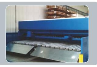
2-axis Back Gauge, X1-X2, for angle cutting
