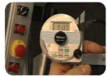
Manually measuring the bending angle and Bending Program Correction
