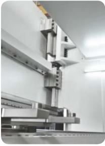
Beam movement on heavy-duty bronze sliders to secure safety and accuracy
