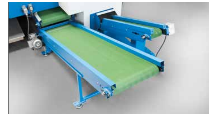
Double conveyor to unloading point
