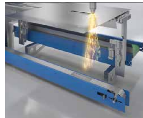
Standard conveyor for disposal of slag and waste of sheets
