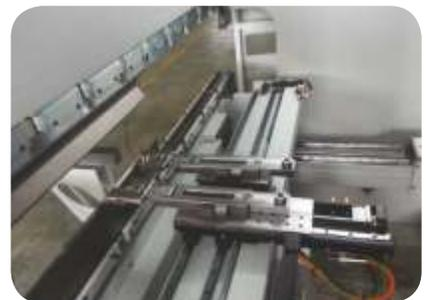
5-axis high-speed back-gauge system, X'-R-Z1-Z2
