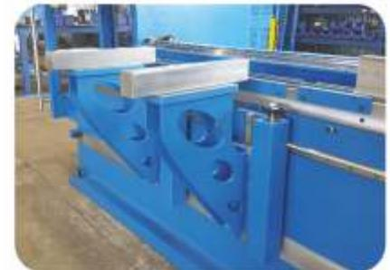
Moveable heavy-duty front supports on linear guide
