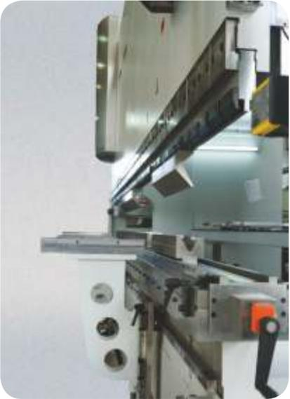
Heavy-duty clamping system up to 350t/m (optional)
