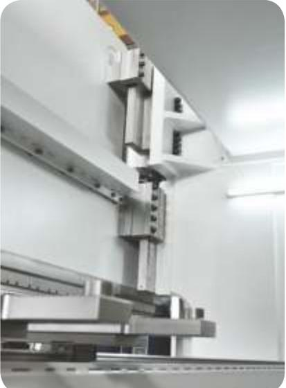
Beam movement on heavy-duty bronze sliders to secure safety and accuracy
