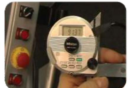
Manually measuring the bending angle and Bending Program Correction
